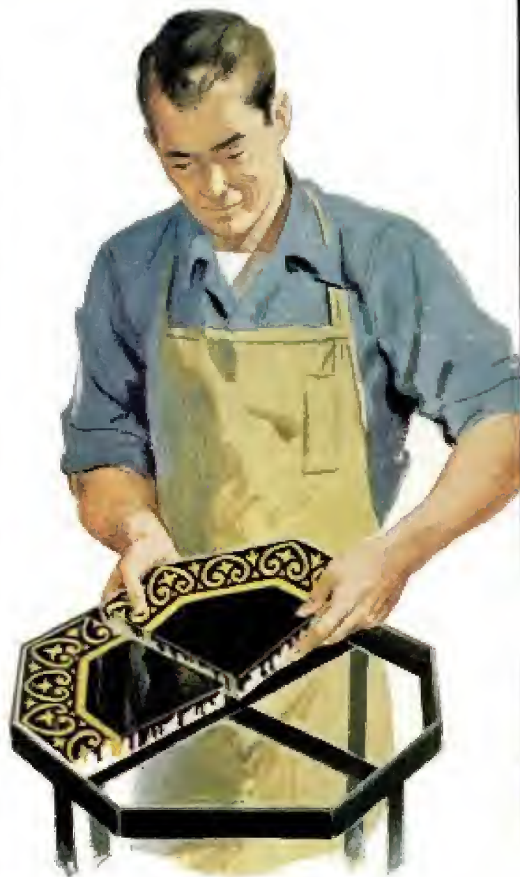
Illustration above shows tile being checked for proper clearance in steel-angle table frame. Hexagonal frame and base were made as in the detail below
